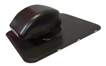
Prior to installation, the 4" duct drop connector must be field assembled to the main vent assembly as shown on the carton instructions and illustrations. This is a simple operation, just align and press to snap into place, then check to ensure a proper connection is achieved. Duct connections can be made from the roof if the duct can be accessed through the roof during installation, if not then attic space access by the installer will be required.
