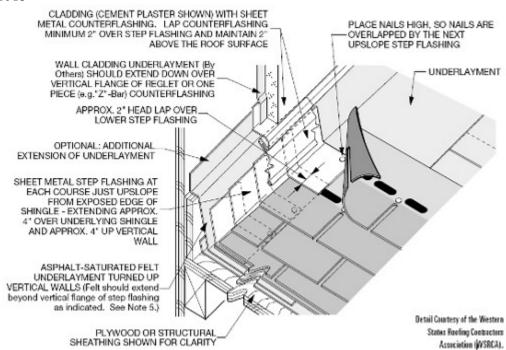
Proper flashing is a critical component of all roof systems. On steep-slope shingle applications, flashings at vertical intersections are completed with metal step flashings. Step flashings should be fabricated from a non-corrosive metal such as minimum 24-gauge galvanized metal or 16-ounce copper.
