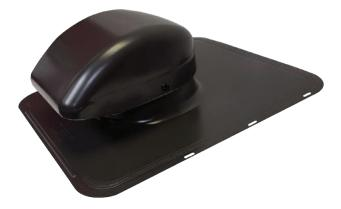
Prior to installation, the 4" duct drop connector must be field assembled to the main vent assembly as shown on the carton instructions and illustrations. This is a simple operation, just align and press to snap into place, then check to ensure a proper connection is achieved. Duct connections can be made from the roof if the duct can be accessed through the roof during installation, if not then attic space access by the installer will be required.
